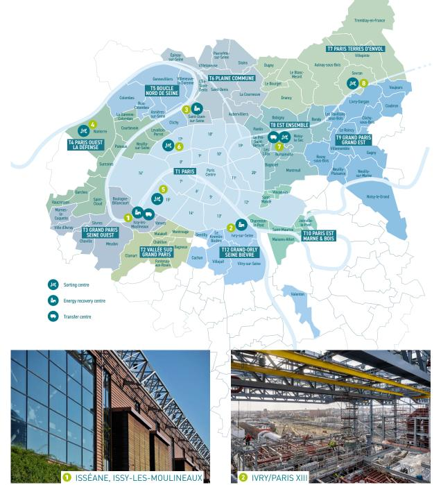
• Energy recovery unit Catchment area: 1.3 million inhabitants 521,650 tonnes incinerated in 2021 Authorised capacity: 520,000 tonnes Operator: Issy Urbaser Energie • Energy recovery unit Catchment area: 1.4 million inhabitants 709,713 tonnes incinerated in 2021 Authorised capacity: 730,000 tonnes Operator: IPXIII (Suez)
