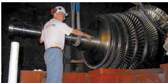
Turbine generator at the Isséane centre
