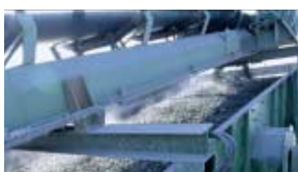
The clinker conveyor belt at Saint-Ouen-l'Aumône.
