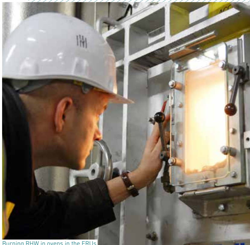
Burning RHW in ovens in the ERUs produces energy.
