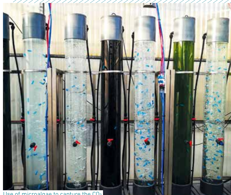
Use of microalgae to capture the CO 2 contained in incineration flue gases.
